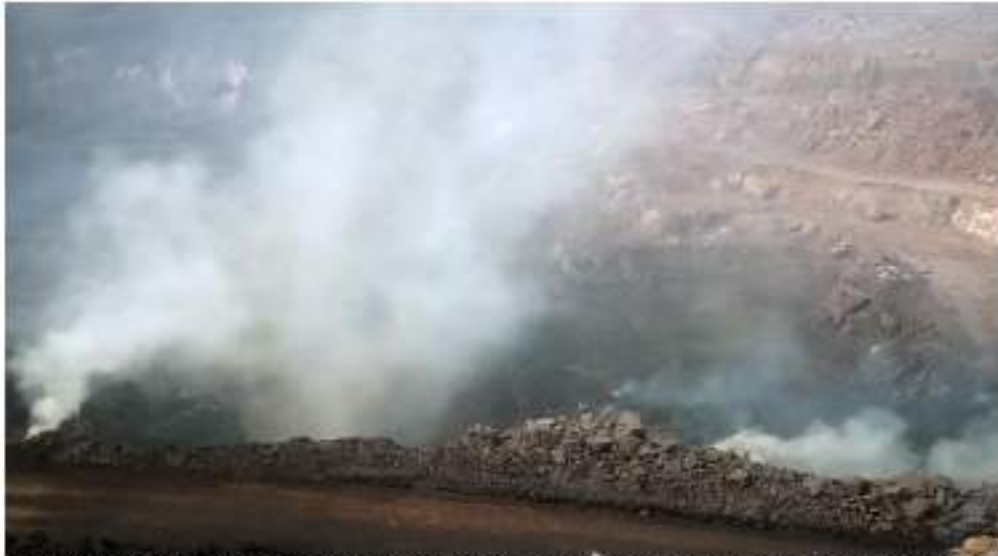
Figure 17: Coalfries in active seams in Kusunda (point 23 in figure 13 and table 4)
