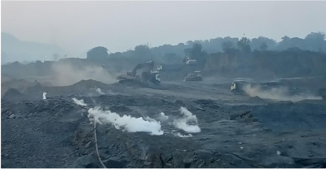
Figure 19: Fire in OB dumps in Kusunda area. (point 24 in figure 13 and table 4)
