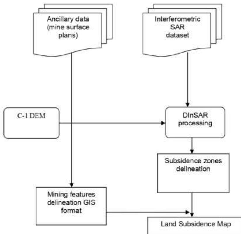
Figure 7. Work flow diagram for generating land subsidence map using DInSAR technique.
