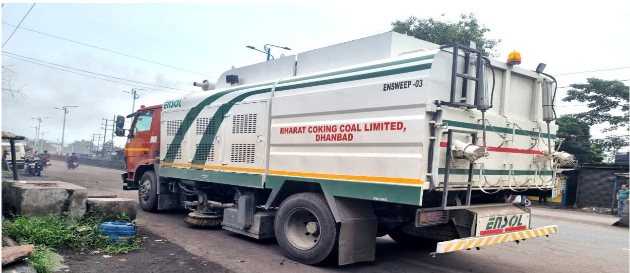
Mechanical Sweeper in Bastacolla Area
