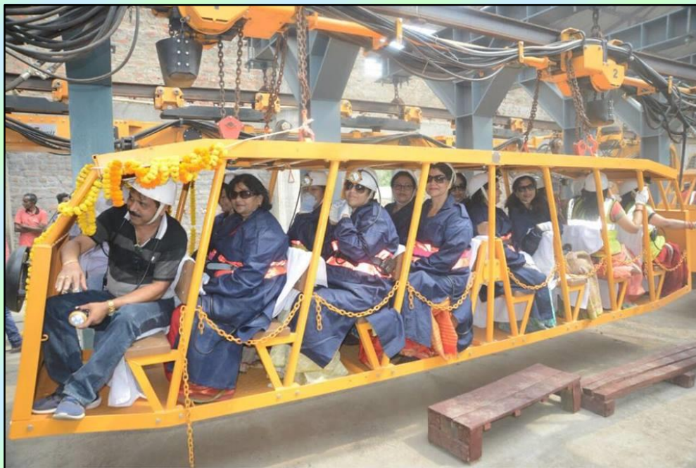
For the first time in India in underground mines, suspended-diesel-hydraulic monorail locomotive system has been installed in Moonidih XV Seam Incline No. 1, BCCL as an equipment for man riding and material transport.
